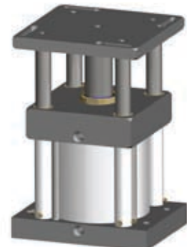
Lifter 4 Post. Ex: 5" bore, 4" stroke, main rod 1.75" dia and the 4 post at 1" dia. The post are garded by thin wall tubing.
