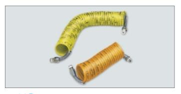
Legris nylon recoil tubing ensures that the coil will continue to contract after multiple use. Assembled with male connector 1/4" BSP taper fittings, it is ready for immediate use. Protection springs are fitted to prevent the ends of the tubing from becoming damaged.
