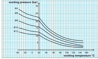
To calculate burst pressure, the values in the above graph should be multiplied x 3. (For flow chart information on fractional inch, please
