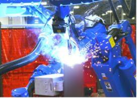
Electromagnetic fields are common to the welding process can cause standard inductive sensors to fail. Fortunately, the Contrinex **DW-661** and **DW-673** series feature magnetic-field-immune electronics that allows the sensor to function without false signals in these environments, ensuring accurate Factor 1 detection of steel and aluminum sheetmetal targets.
